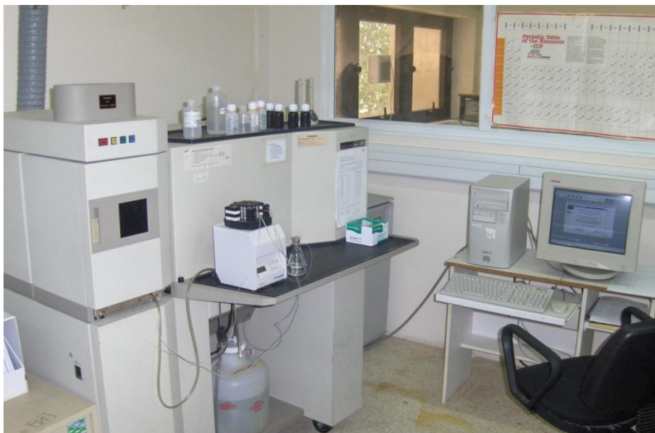
Photo 3.12: ICP-AES instrument used for heavy metals analysis
