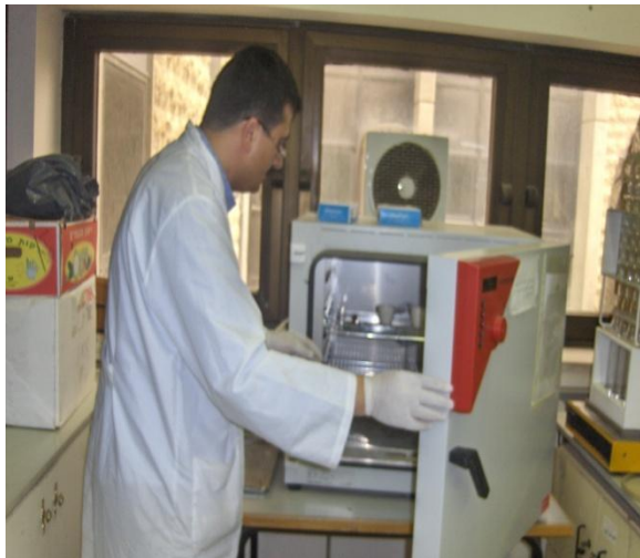
Photo 3.4: Incubating Biosolids samples in furnace at 105 °C
