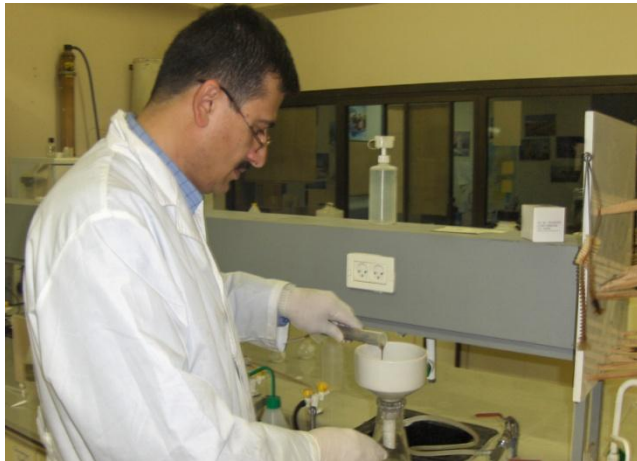
Photo 3.6: Suspended solids determination through suction filtration of sludge sample
