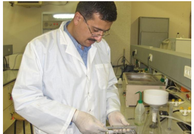
Photo 3.7: The suction setup ready to start sample filtration
