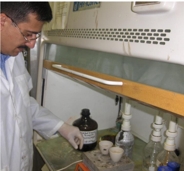
Photo 3.10: Biosolids sample digestion on a plate heater
